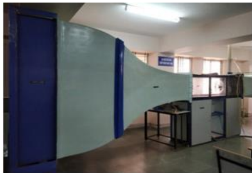
Figure 3. Wind tunnel test rig with scaled bus model
